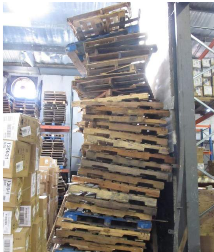
Figure 35.1: Unsafe Pallet Storage in Panama
